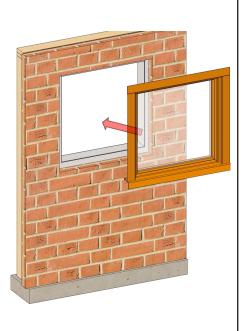
Install window into opening, making sure window is square and plumb. Refer to standard QWP installation guide.
