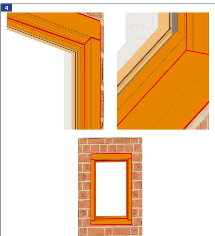
Clean panning where sealant is going to be applied. Apply sealant to all seams and remove excess from exterior of window. Shown above, sealant where panning meets panning, and sealant where panning meets exterior of the window and corner seams.
