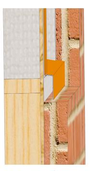
Note: If needed, rip exterior leg of panning to properly fit the masonry opening. As shown above the bottom of the panning is ripped in order to fit flush with the brick wall.
