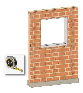
Measure and verify the size of the rough opening, making sure each side is level, shim if needed.
